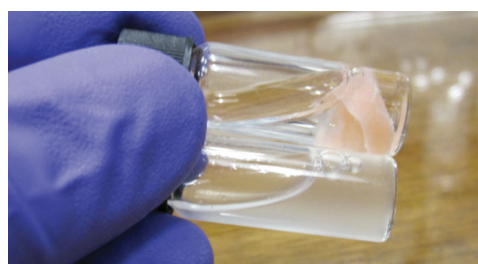
Figure 4. The formed CNC-g-P(DMAEMA- r -NpMA)/PVA-MV/CB[8]-based hydrogel (top sample, for composition, see Table 1, entry 1) and the control sample (bottom sample) that contained the first and second guest functional components (CNC-g-P(DMAEMA- r -NpMA) and PVA-MV) at similar composition without CB[8] – note the absence of red colour and any precipitate formation. Also, note the change in volume and the clear supernatant in the top sample due to centrifugation step.
